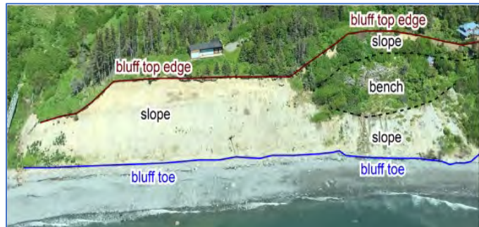
Image of a coastal bluff erosion with delineated toe/bottom (blue) and top edge (maroon) with slope area in between. (DGGs)
