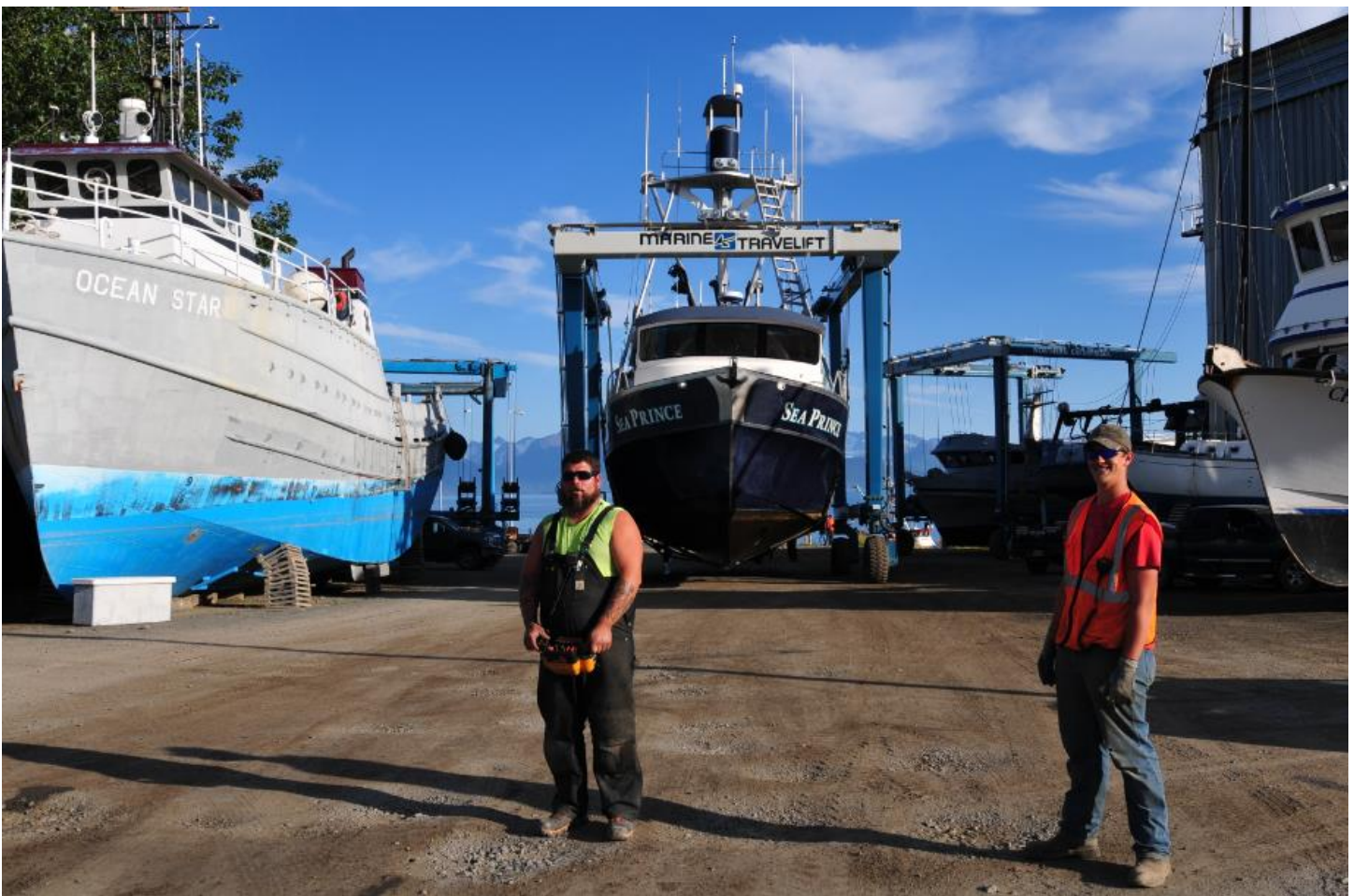
This picture was taken this fall. The Sea Prince was built in our yard several years ago and is coming back in for a paint job and small work. It is Fiberglass, 58 by 20. Two of our crew in front, Aaron and Blade. The vessel on the left, The Ocean star, had to be lightened for us to lift it and It is getting a major refit, from some sort of cargo to a fishing tender.
