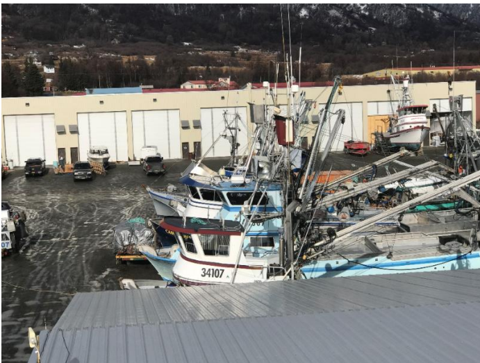
This building is 204 feet long with 8 bays, 25 by 60 each. All are full, a boat in each. We will roll as many in and out as the time allows before summer. On the right is a seiner being lengthened out to nearer 58 feet. The bow you can see in the other bay is a 53-foot charter boat from Seward, getting a complete over haul. Its sister ship was done last winter.
