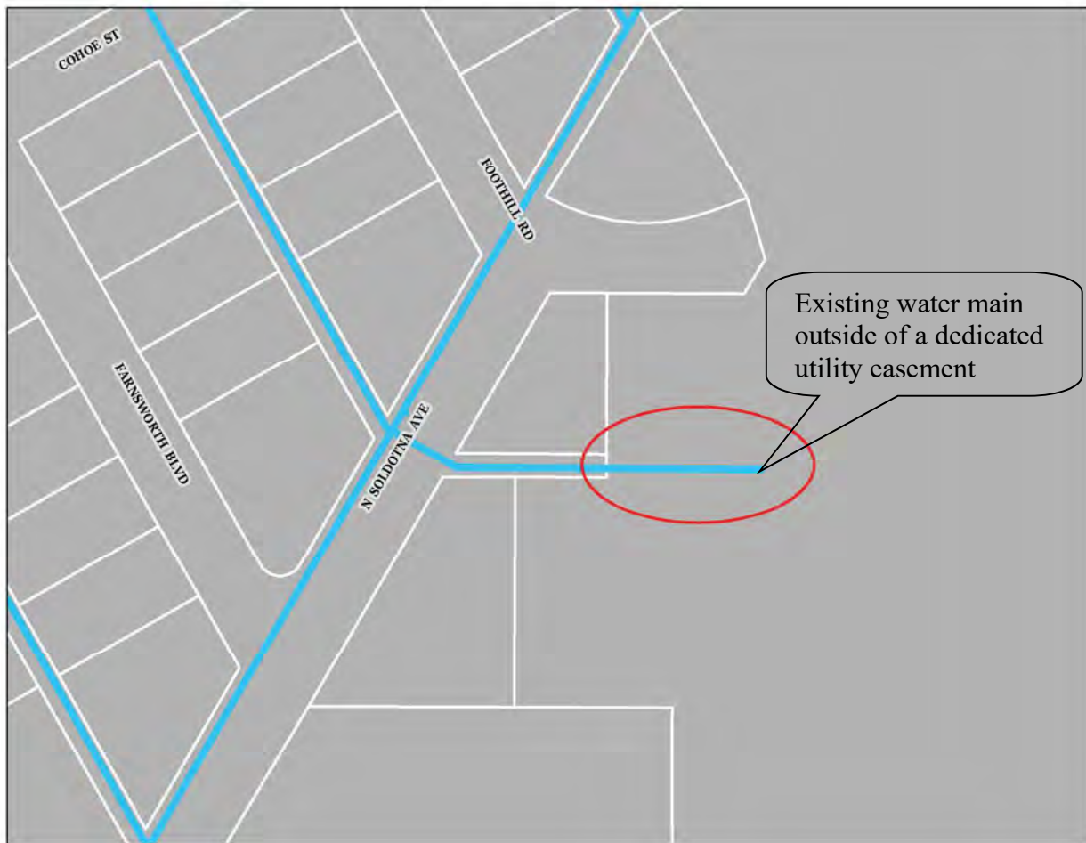
Figure 5. A portion of a water main is within the 20-foot wide electrical distribution line easement.
