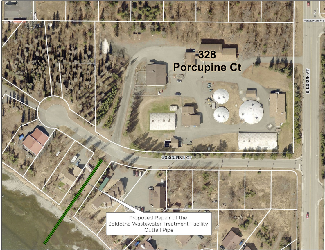
Figure 1. Proposed site for the repair of the outfall pipe from 328 Porcupine Ct.
