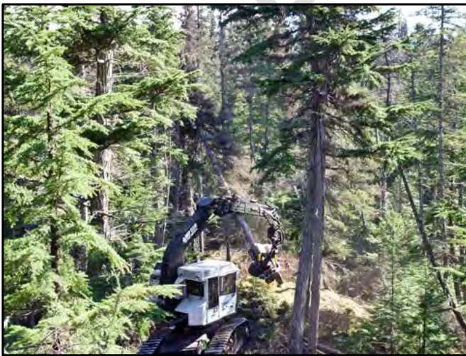
Figure 4.15. Feller buncher used to remove whole trees.
