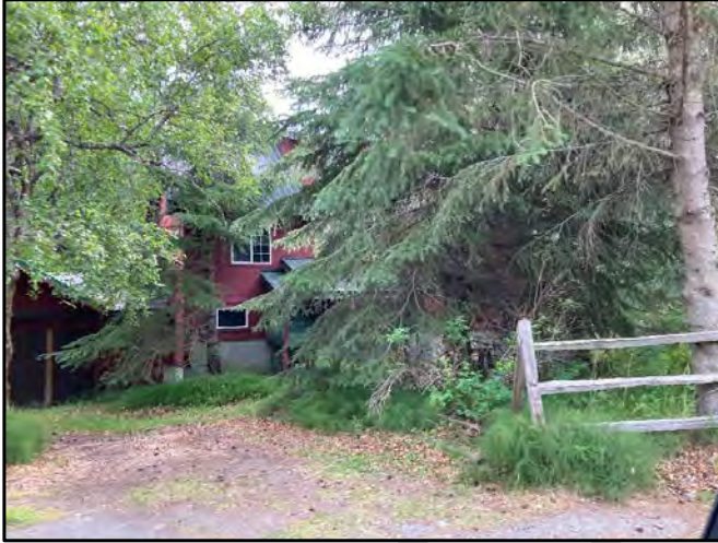
Figure 4.7. Example of poor defensible space.
