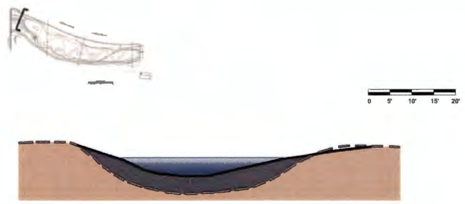
Figure 7. Cross Section of the Outlet Stream Channel Fill and gravel is added to create a stream channel with salmon spawning habitat.
