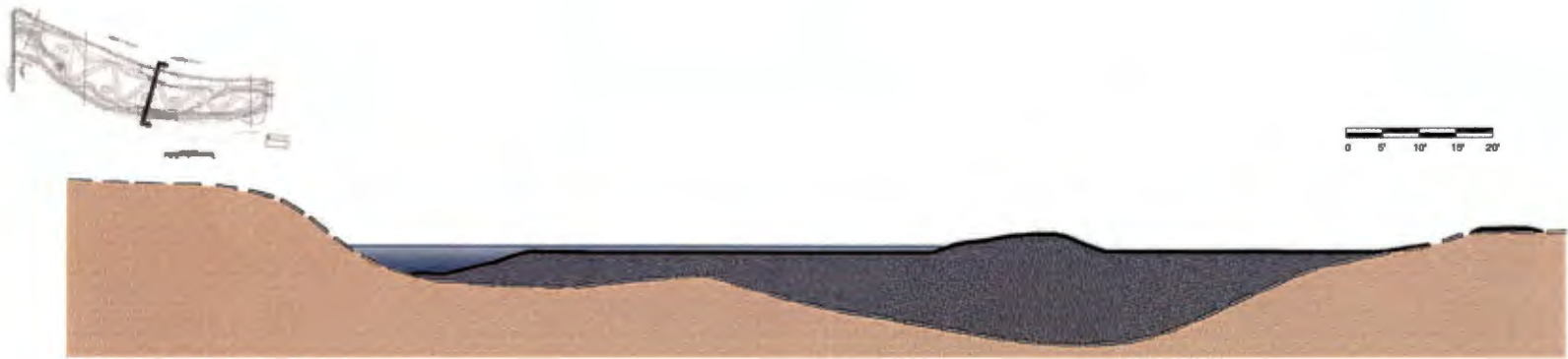
Figure 5. Cross Section of the Stream Channel, Marsh, and Island Fill is added to create wetland emergent plant zones. The upland island will create protected bird nesting habitat.
