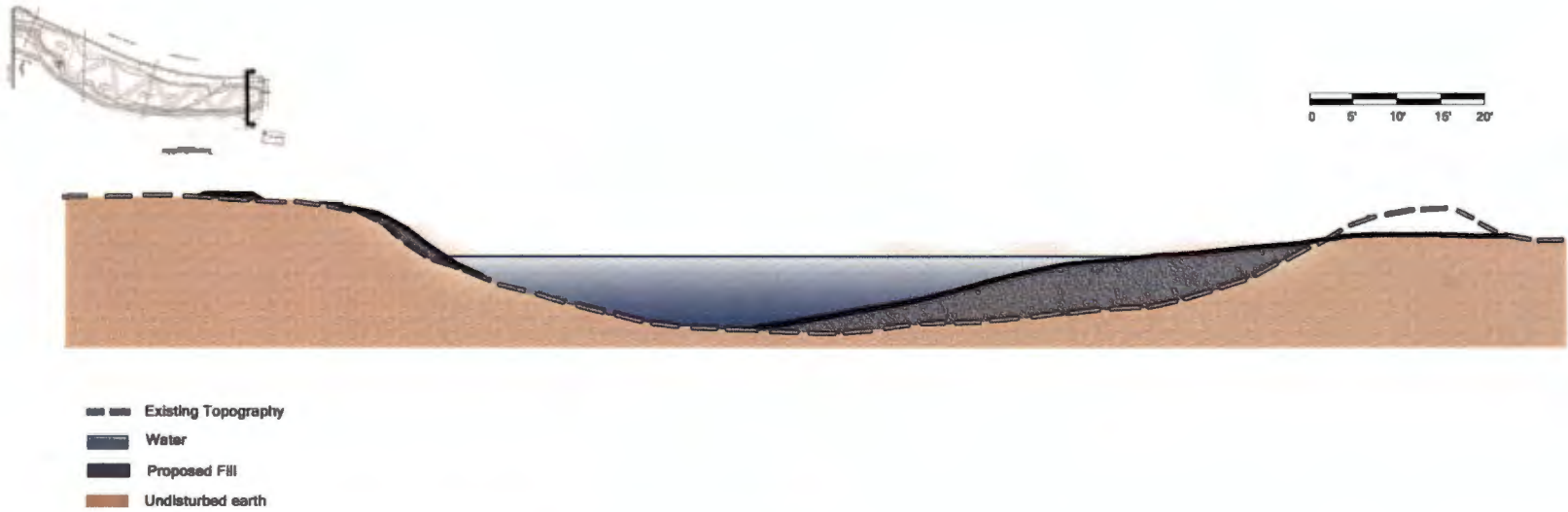
Figure 4. Cross Section of the Coho Salmon Overwintering Pond Fill is added to modify the steep wetland edge and cut is removed to allow the truck hauling road for the construction phase.
