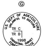
Found standard USDA Forest Service 2 1/2" diam. alum. post, with 3 1/4" diam. alum. cap, 3" above the ground, mkd. as shown, from which,
