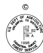
Found standard USDA Forest Service 2 1/2" diam. alum. post. with 3 1/4" diam. alum. cap, 9" above the ground, mkd. as shown, from which,
