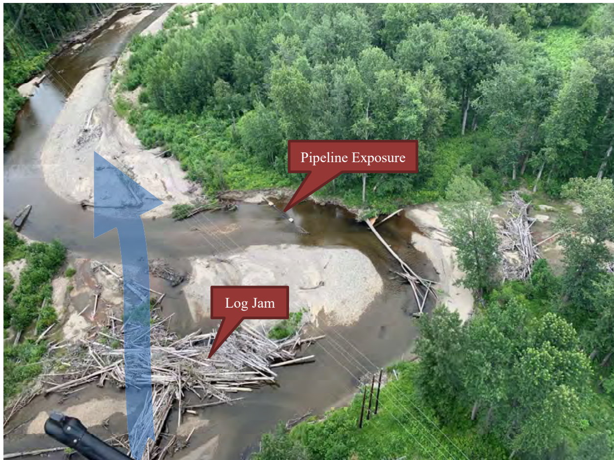
Photo 1. Exposed Beluga Pipeline in Chuitna River; photo taken facing east on July 17, 2020. Blue arrow depicts the original river channel.
