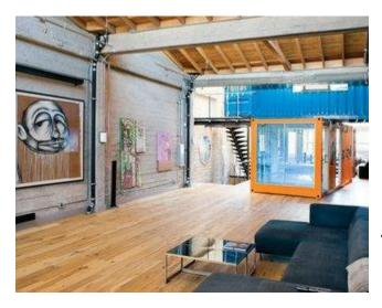
Two San Francisco art and travel addicts overhauled a loft—and customized a pair of shipping containers—to accommodate their collection and reflect their passions. The shipping containers were stacked, joined with steel tubes, and lashed to reinforced floor joints to make them earthquake-safe.
