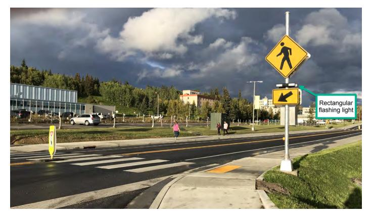
Figure 21: Electrical Warning Devices (Rectangular Rapid Flashing Beacon, or RRFB) on University of Alaska Fairbanks Campus
