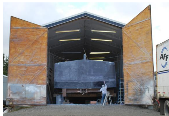
A 58-foot mold being built a few years ago.
