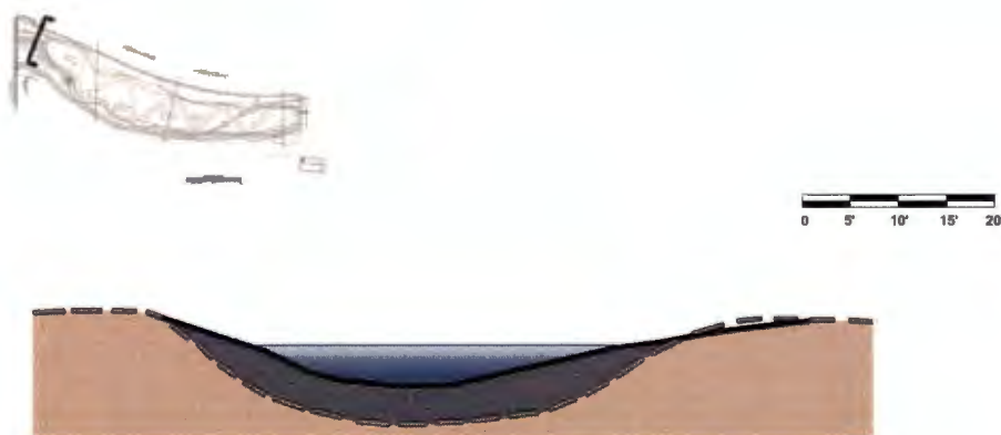
Figure 7. Cross Section of the Outlet Stream Channel Fill and gravel is added to create a stream channel with salmon spawning habitat.
