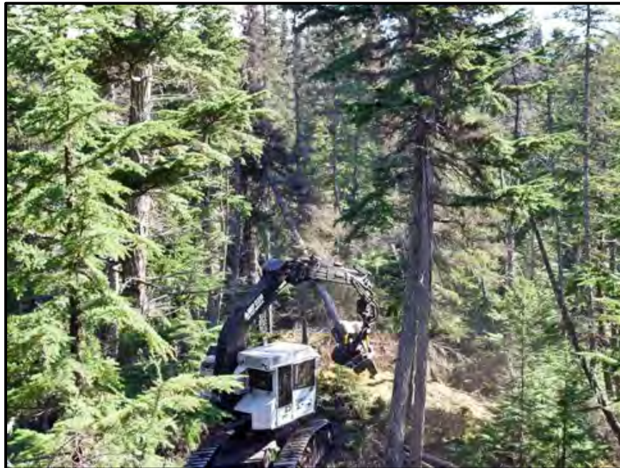
Figure 4.15. Feller equipped with a full-tree processing head that fells, delimits, and then cuts tree stem to desired length or diameter log size.
